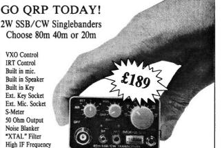
Xtal Fitted gives 3.525-3.550 or 7.075-7.100 or 14.20-14.25MHz depending on model. Virtually no drift! Additional xtals in stock.
