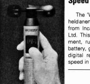
The 'Windy' is a handheld an emometer available from Incastec Associates Ltd. This compact instrument, running on a PP3 battery, gives an accurate digital readout of windspeed in knots or metres/ sec (switchable) with comparison scales for Beaufort or kmh.
